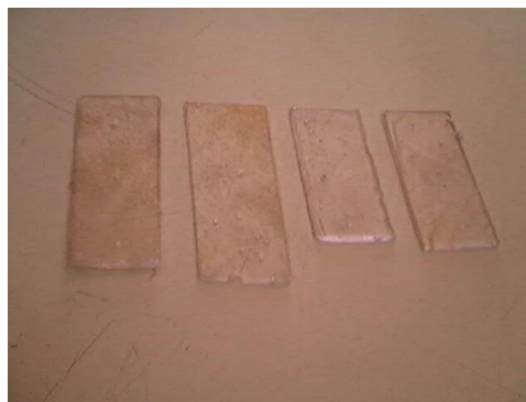
Figure (3.11) effect of number of recycles on appearance (number of the recycle increase to left).
