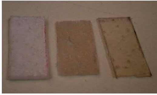
Figure (3.9) effect of temperature on the appearance of the sheet samples in part B (temperature increases to right).
