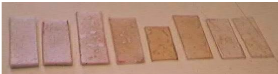
Figure (3.8) effect of temperature on the appearance of the in part A (temperature increases to the right).
